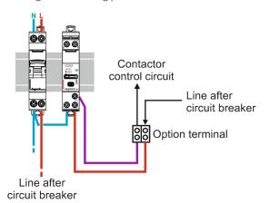
. Control of a single line standard contactor (>20A):
