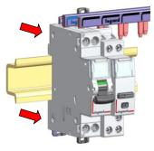
2. Unscrew the terminals and pull the device forward in order to release it from the DIN rail
